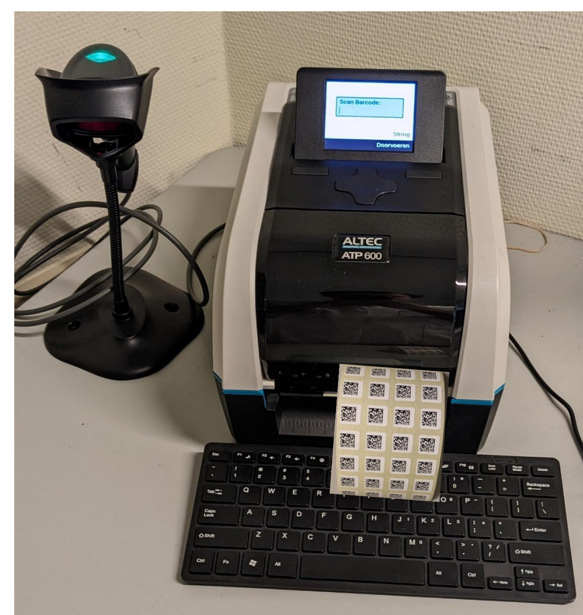
Picture 3: Stand-alone barcode duplicator By scanning the FMD-code on the original package, duplicate 2D-barcodes are generated and printed. FMD-codes include article number (GTIN), expiration date, serial number (for FMD) and lot-number.
