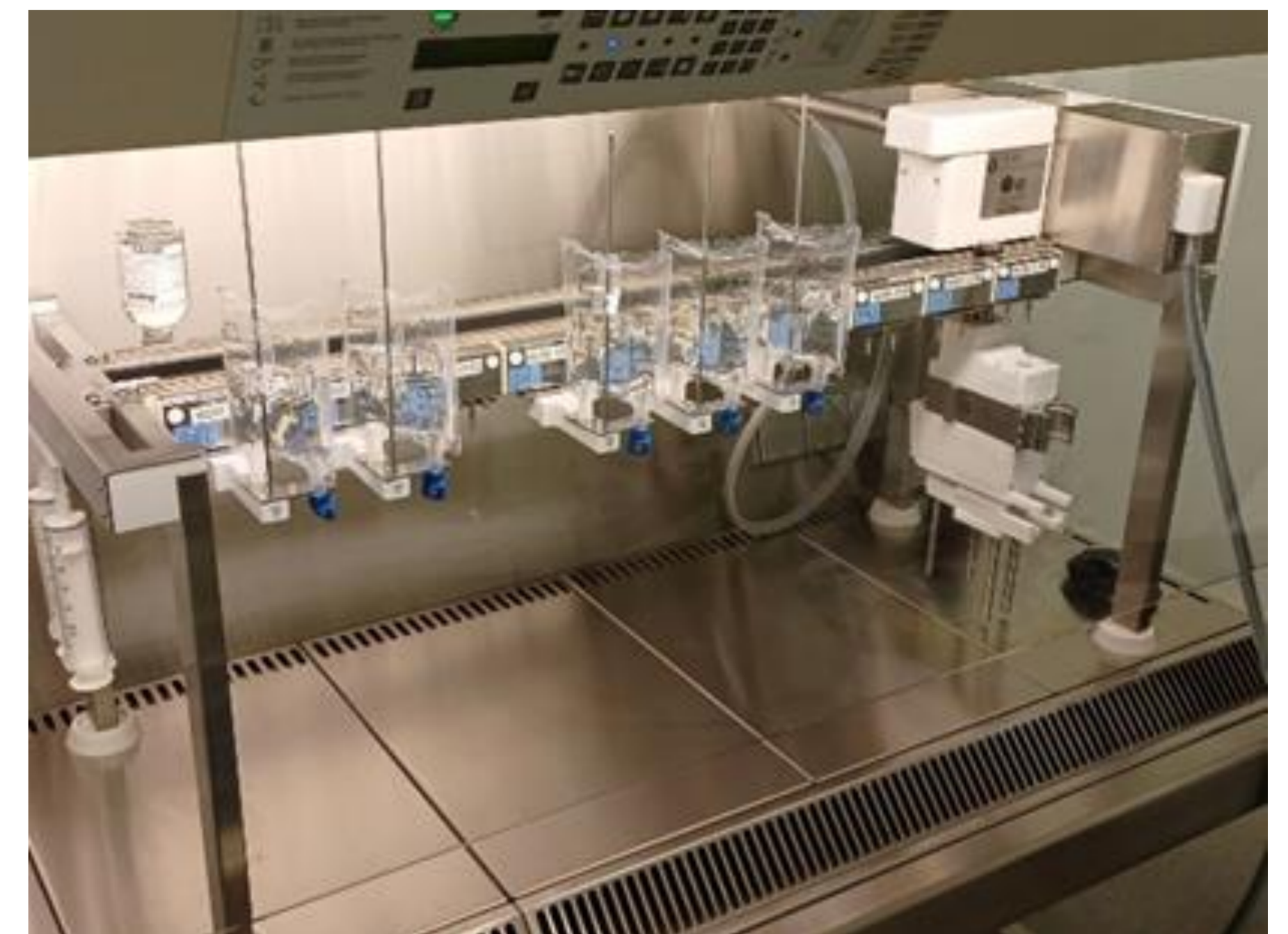
Pic. 1 Holders with infusion bags connected at the front of the device, holders with vials at the back. Syringe fixing position on the left, robot head on the right.
