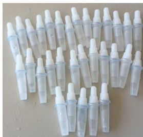
Image 2: Vials after oat-water tightness test.
