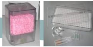
PillBox / PhialBox Locked canisters for loading of medications into packaging station
