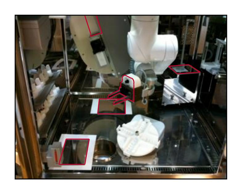
The contamination level of 5 predetermined areas inside the CytoCare<sup>TM</sup> cabinet was investigated with swab tests.
